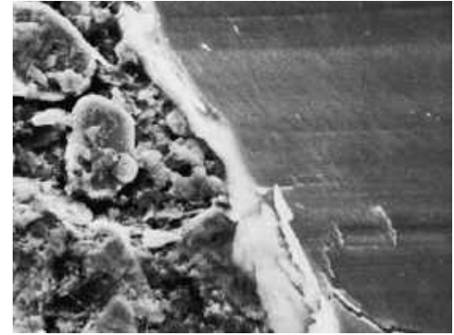
SEM photograph with 1000x magnification: MoS 2 Anti-Friction Coatings before (left) and after (right) load application
